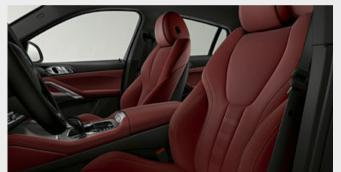
■ Dynamic and comfortable: the standard and individually adjustable Sport seats for the driver and front passenger feature numerous electric adjustment options, including backrest width and seat angle. Together with adjustable thigh support, the taller seat and backrest bolsters provide excellent ergonomics and more lateral support during fast cornering.
