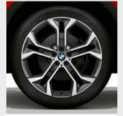
$\square$  21" light alloy wheels Y-spoke style 744 Bicolour Orbit Grey with mixed tyres and runflat tyres\*, gloss-lathed, front 9.5J x 21 with 275/40 R21 tyres, rear 10.5J x 21 with 315/35 R21 tvres.
