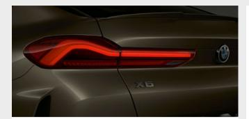
■ The rear lights are made up of individual high-performance LED lighting elements. They have the characteristic, striking BMW L-shape, meaning that the vehicle is clearly recognisable as a BMW even in the dark.
