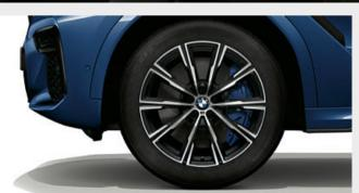
$\blacksquare$  20" M light alloy wheels Star-spoke style 740 M Bicolour Orbit Grey with mixed tyres and runflat tyres, gloss-lathed, front 9J x 20 with 275/45R20 tyres, rear 10.5J x 20 with 305/40 R20 tyres.
