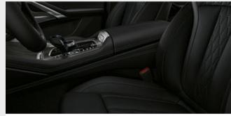
☐ In warm weather, the Active seat ventilation, front\* provides a cool and pleasant seat temperature, resulting in a more comfortable driving experience. Air vents in the seat surfaces and backrests suck air. The intensity of the airflow can be adjusted. The perforated surfaces are made of leather 'Vernasca'.
