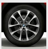
■ 20" light alloy wheels V-spoke style 738 Bicolour Ferric Grey with mixed tyres and runflat properties\*, gloss-lathed, front 9J x 20 with 275/45 R20 tyres, rear 10.5J x 20 with 305/40 R20 ty-
