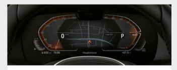
■ The BMW Live Cockpit Professional with navigation function¹ includes two high-quality displays consisting of a high-resolution 12.3" Control Display that can be operated by touch and a fully digital 12.3" instrument display
