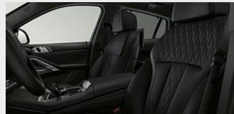
☐ The comfort seats for driver and front passenger include active headrests and can be electrically adjusted in various ways. The top part of the backrest, the backrest width, thigh support and headrest height can be individually adjusted. The equipment package range also includes the lumbar support and memory function for the driver.
