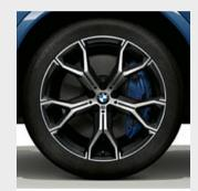
$\square$  21" M light alloy wheels Y-spoke style 741 M Bicolour Orbit Grey with mixed tyres, gloss-lathed, front 9.5J x 21 with 275/40 R21 tyres, rear 10.5J x 21 with 315/35 R21 tyres.<sup>2,3,6</sup>
