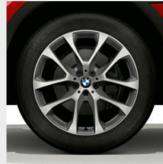
■ 20" light alloy wheels V-spoke style 738 Bicolour Ferric Grey with mixed tyres and runflat properties, gloss-lathed, front 9J x 20 with 275/45 R20 tyres, rear 10.5J x 20 with 305/40 R20 tvres.
