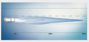
☐ **BMW Laserlight** in a unique X design reaches a maximum illumination range of up to 500 m in laser high-beam mode.
